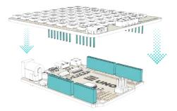
Once connected, the Glow UNO can be powered through the UNO or via the onboard USB C power port. For optimal performance, especially when driving a large number of LEDs at high brightness levels, it is recommended to use an external 5V power supply through the PD compatible USB C port on the shield. Using this port will also power the UNO board.
